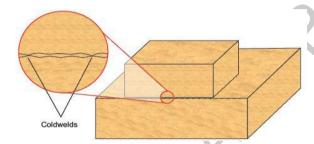
The contact points between the two surfaces form a sort of cold welds. These cold welds resist the surfaces from sliding over each other. Adding weight over the upper block increases the force pressing the surfaces together and hence, increases the resistance. Thus, greater is the pressing force greater will be the friction between the sliding surfaces.
