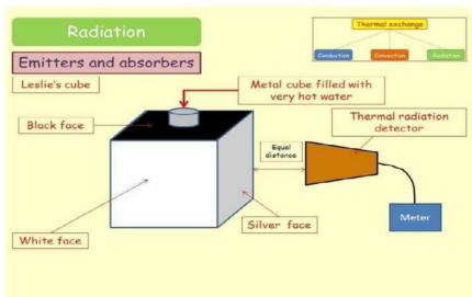
Hot water is filled in the Leslie's cube and is placed with one of its face towards a radiation detector. It is found that black dull surface is a good emitter of heat. The rate at which various surfaces absorb
