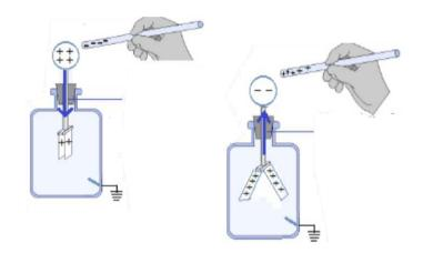
iii. Investigating whether the body under test is conductor or insulator.
